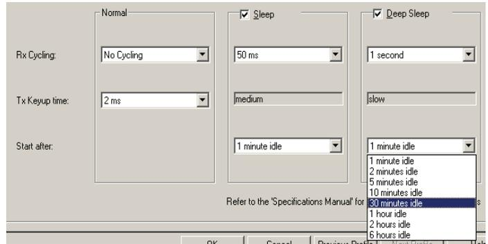
In Deep Sleep mode, the receiver cycling time can be as slow as one second. The TB8100 switches off the PMU DC-DC converter and runs using the standby power supply module. Because the highly efficient standby supply provides 10W and only powers the reciter, power savings are dramatic.
